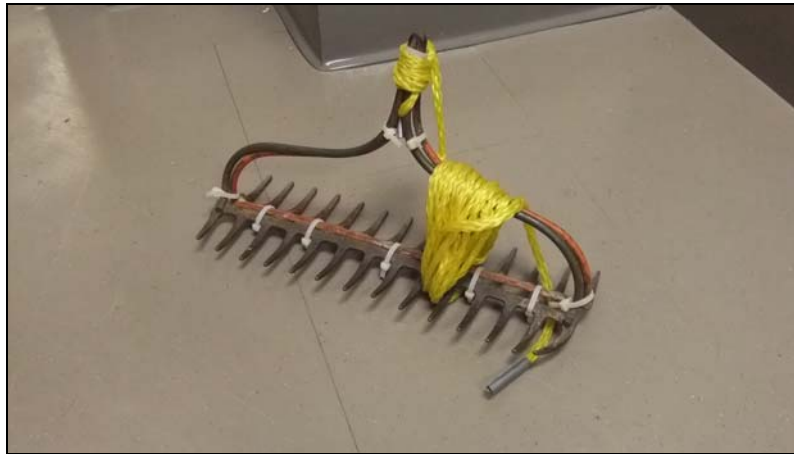
Figure 2. Double headed rake used to search for aquatic plants in deep sections of the Eno River.
